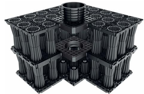
Please ensure the access plate is not used on the edge of your system! The remote access plate must be used at least one module inside from the perimeter of you system. Also the remote access plates cannot be placed next to each other as the protruding lip around the top edge will prevent this, again please ensure at least one StormBrixx module is placed between them.
